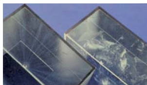
Figure 2.2.2 Left : Streaks due to moist granules Right : Streaks due to moisture on the mould surface
