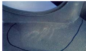
Figure 2.3.1 Air streak due to entrapped air
