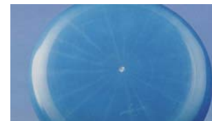
Figure 2.4.4 Streaks around primary and secondary weld lines
