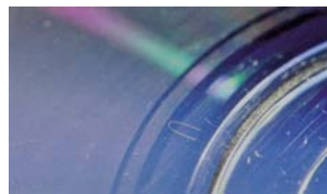
Figure 2.3.2 Streak (near the gate) due to air drawn in during decompression
