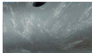
Figure 2.3.2 Streak (near the gate) due to air drawn in during decompression
