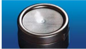
Figure 1.3 - Sink marks on a cylindrical core with poor temperature control
