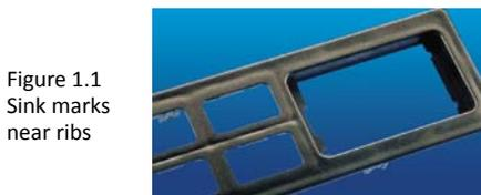
Figure 1.1 Sink marks near ribs
