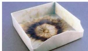
Figure 2.1.1 - Charred streaks due to on excessive residence time in the hot runner / plasticising cylinder
