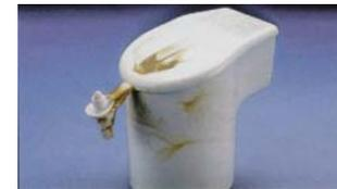
Figure 2.1.3 - Charred streaks due to an excessive residence time in the plasticising cylinder
