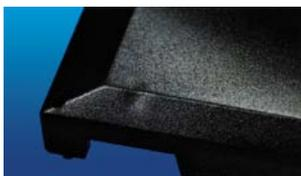
Figure 1.2 Sink marks near a dome
